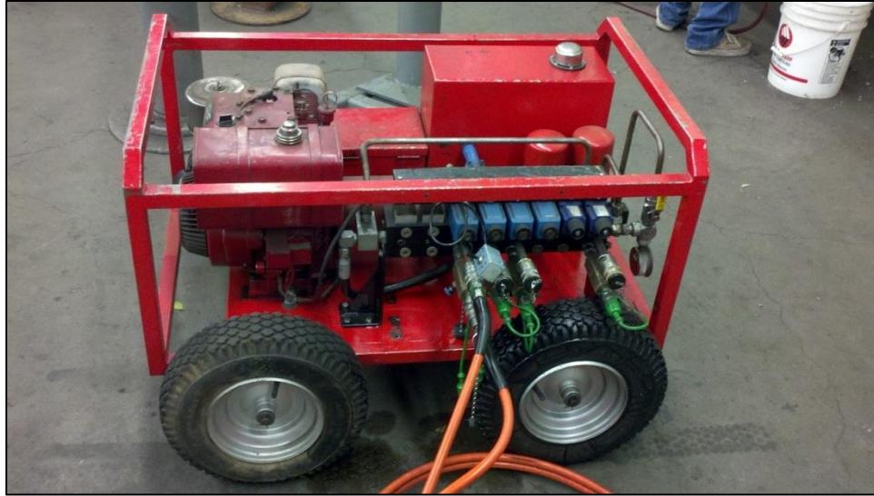
Figure 23. BRAE Hydraulic Power Pack.
