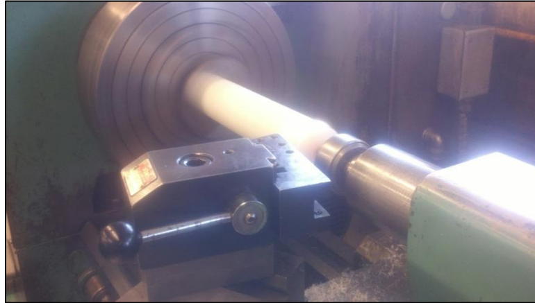
Figure 20. Machining the UHMW Bushings with the Lathe.
